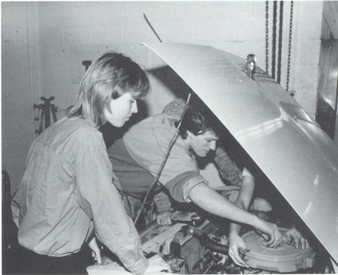
Sophomore Allan Kroenke and Craig Cabble are carefully replacing the carburetor in the engine.
